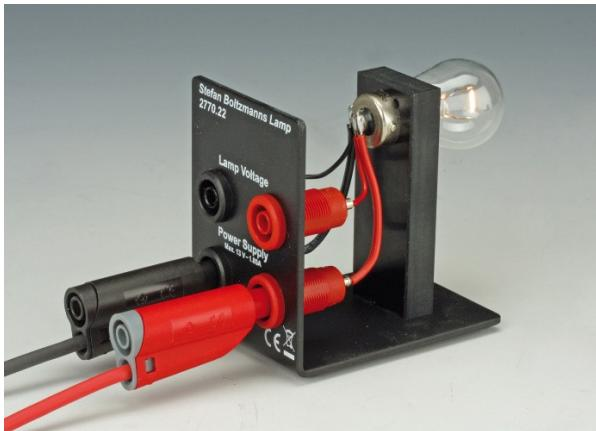
The Stefan-Boltzmann Lamp is equipped with a filament of tungsten.
