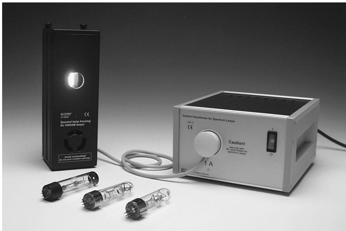
The control transformer is the power supply for our spectral lamps. The spectral lamps changes the internal resistance when they are heated (during use), which demands a special type of power supply. Thus it is necessary to reduce the current, when the internal resistance is low. Therefore the control transformer is especially designed to reduce the current in the lamp to Max. 1 Amp.
