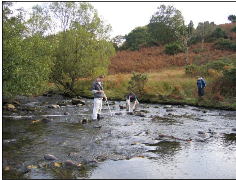
Figure 7 Measuring “Distance Out” using tape secured at each end
