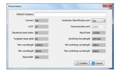
User can view the parameters and modify the Company name. Whether choose the Automatic Identification port or not also can be set up. Finally, click the button confirm to exit the parameters window. User also can close the window directly without any modification.
