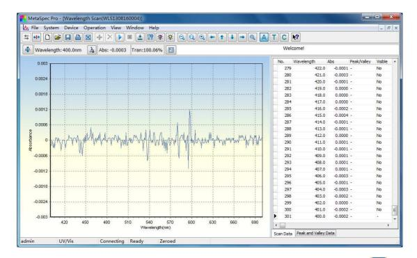
5. After the measurement is completed, click the shortcut icon the toolbar to save the test data. The file will be saved in "WLS" format. Click the shortcut icon in the toolbar to print the test report. The data also can be exported to Excel by clicking the shortcut icon in the toolbar.
