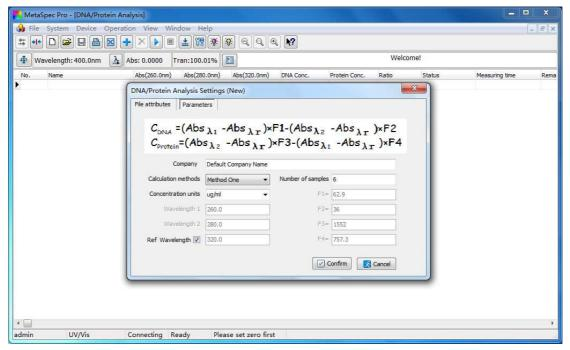
2. Select the Calculation methods, Concentration units and choose whether calibrating with "Ref Wavelength" or not. Input the
