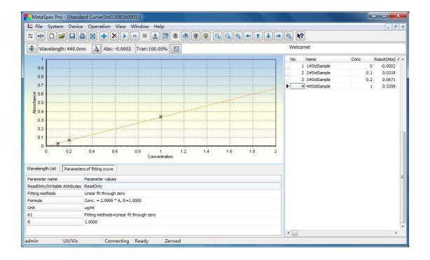
7. After the measurement is completed, click the shortcut icon line the toolbar to save the test data. The file will be saved in ".Std" format. Click the shortcut icon line in the toolbar to print the test report. The data also can be exported to Excel by clicking the shortcut icon line in the toolbar.
