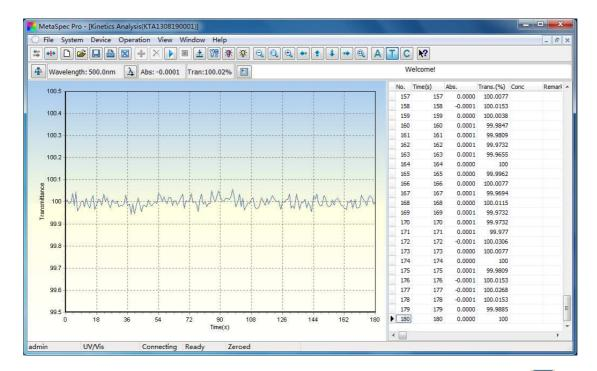
5. After the measurement is completed, click the shortcut icon in the toolbar to save the test data. The file will be saved in "KAT" format. Click the shortcut icon in the toolbar to print the test report. The data also can be exported to Excel by clicking the shortcut icon in the toolbar.
