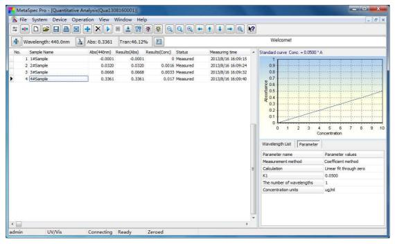
6. After the measurement is completed, click the shortcut icon line the toolbar to save the test data. The file will be saved in "Qua" format. Click the shortcut icon line in the toolbar to print the test report. The data also can be exported to Excel by clicking the shortcut icon line in the toolbar.
