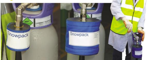
The Snowpack makes individual pellets of dry ice from a carbon dioxide syphon cylinder, which has an internal dip tube.
