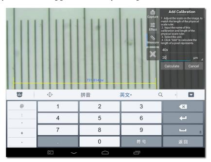
2. Input the name of the calibration and the physical length of the ruler. We input 40x for the name, that means the magnification of objective is 40X,
