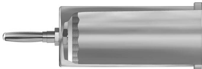
The bullet catcher is used for investigating the conservation of momentum. It is mounted at the ends of a glider for the air track. The set contains two bullet catchers in order to preserve the balance of the glider.
