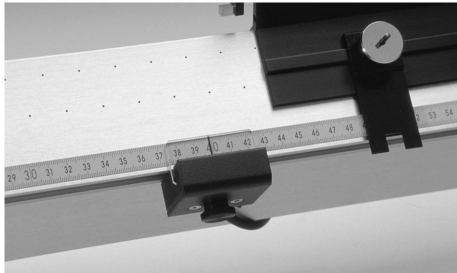
The photocell can be described as an optical switch which is activated when the light beam is blocked. The photocell may also be activated when the light beam again is uninterrupted.
