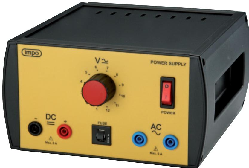
The power supply no. 2158.10 provides AC and DC power in 1 volt increments, from 1 to 12 volts, at up to 6 A. As the AC and DC power are delivered on separate output connectors, they may be used simultaneously. Both output are unregulated, and protected from current overload by thermal circuit breaker. The DC output is fullwave rectified, but unfiltered.
