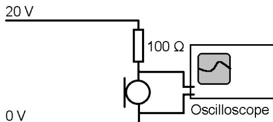
The bias voltage and the load resistor can be changed to vary the dynamic range of the microphone.
