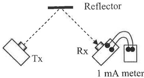
The path length should be  $\sim 1.5\text{m}$ . Switch Tx and Rx on (without horns). Turn Rx gain clockwise, then turn Tx tune until the meter reading goes high (usually off scale). In turn, decrease Rx gain and readjust Tx tune until a full-scale reading where Tx tune is at the maximum position.
