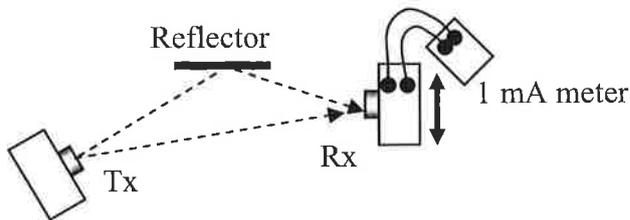
By using a mirror, two incident sound sources can be set up. This creates an interference pattern which can be observed by moving the receiver along the line perpendicular to the reflector.
