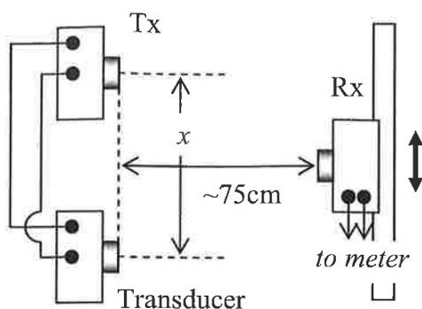
Connect the transducer to the monitor and earth terminals on the transmitter. The transducer will now emit a signal with the same amplitude and phase as the transmitter. (Twin or separate leads are satisfactory up to a separation of 1m). If a meter rule is secured on the bench, and Rx moved up and down it, minima and maxima are observed, the separation of which depends on  $x$  which represents to the distance between slits in a Young's optical experiment.
