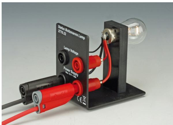
The Stefan-Boltzmann Lamp is equipped with a filament of tungsten.
