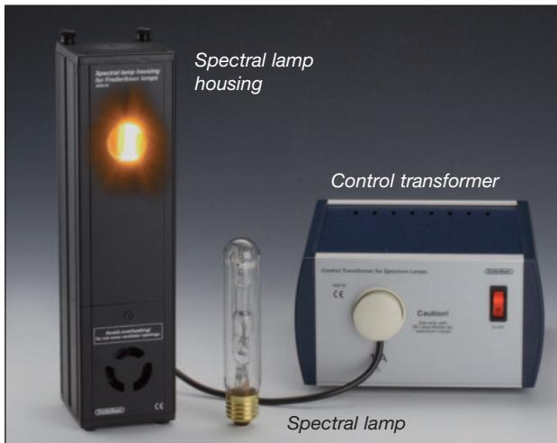
This Spectral lamp house is designed for use with spectral lamps which fit a E-27 socket. These spectral lamps must never be connected to the mains, but require a control transformer, type 2840.50. The Spectral lamp house is equipped with a ventilator ensuring that the surface of the Spectral lamp house does not exceed 60 degree C.
