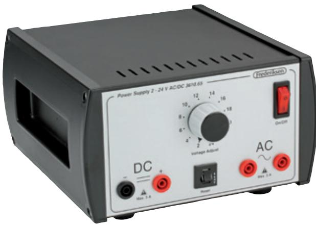
The power supply no. 3610.65 delivers from 2 to 24 V DC and AC voltage and a current of up to 5 A. The voltage can be selected in increments of 2 V.
