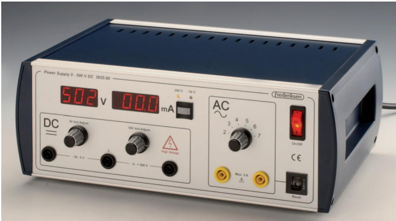
The power supply no. 3655.61 provides a rectified, smoothed, stabilized and regulated DC power in 2 voltage ranges: 0 to -50 V DC and 0 to +500 V DC. The built-in current-limiter limits the current to 50mA, thus protecting the apparatus against shortcircuits in both ranges.
