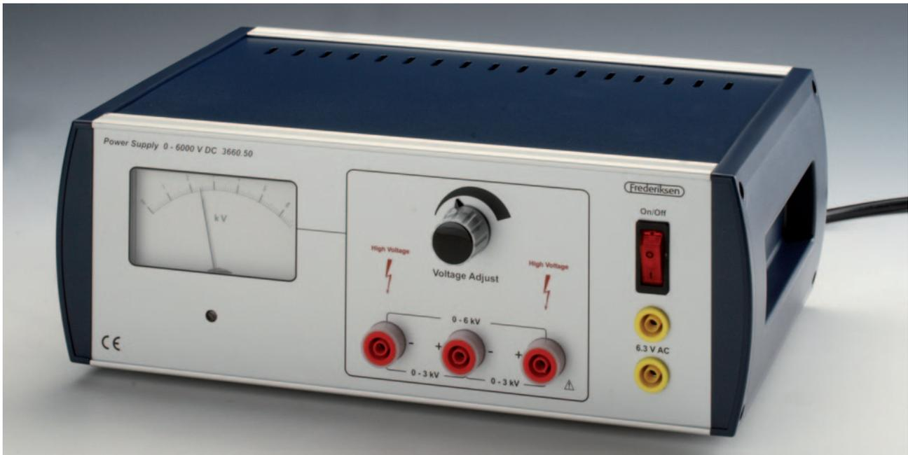
The kilovolt powersupply provides regulated DC power from 0 to 6 kilovolts at up to 2 mA. The 6 kilovolt output also has a center tap, providing outputs of 0 to  $\pm 3$  kilovolts. In addition, the supply output jacks provide a constant 6.3 volts of AC power in electron tube experiments.
