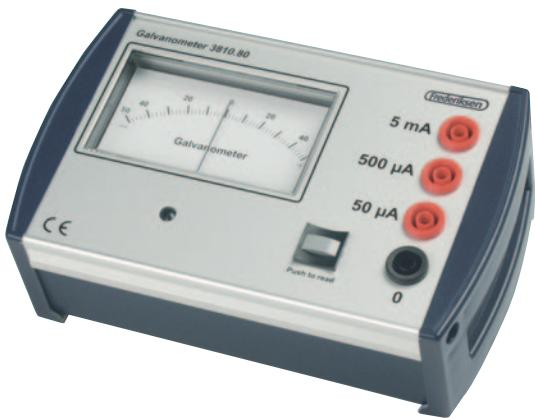
The Student Galvanometer is a rugged yet sensitive instrument, designed specifically for student experiments. It has a center-zero meter and three current ranges. When performing a null-current experiment, such as measuring resistance using a Wheatstone bridge, it is easy to balance the current using the 5 mA range, then step down through the lower current ranges to very accurately determine the point of zero current.
