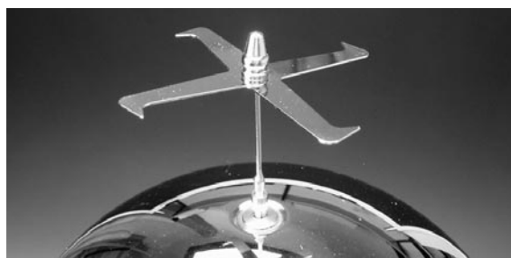
Figure 10: The "electric whirl" apparatus (4430.00) is shown mounted on a Van de Graaff generator (3700.50). When the sphere is charged, the little mill will rotate.
