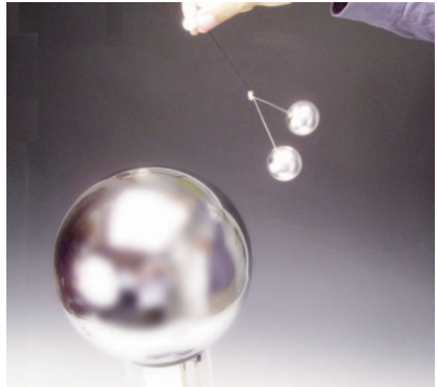
Figure 6: Either a metal sphere (3705.00) mounted on an insulating rod (or the sphere of a Van de Graaff as shown here) is charged. Forces acting on pith balls or metalized balls placed near the sphere indicate the presence of an electric field.
