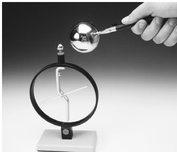
Figure 9: An electroscope (4410.00) is shown. It is acted upon by a charged metal ball on an insulating rod (4415.00).
